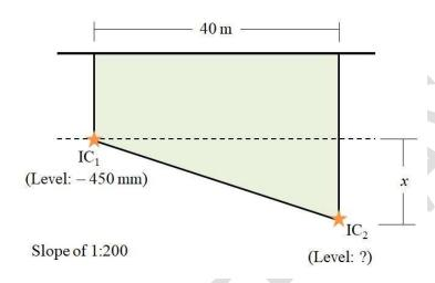
Slope is calculated as (rise/run). Here, rise = x and run = 40 meters = 40,000 mm
